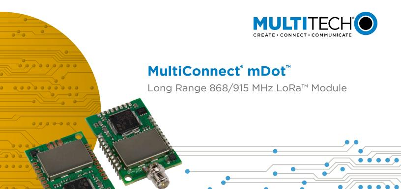
The MultiConnect\* mDot™ is a secure, CE/FCC certified, ARM® mbed™ programmable, low-power RF module, that provides long-range, low bit rate M2M data connectivity to sensors, industrial equipment and remote appliances.
