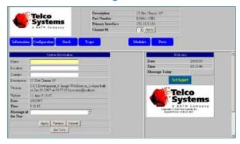
The Metrobility® WebBeacon Element Management System by Telco Systems® is a browser-based element and service provisioning software enabled through an embedded kernel which resides on the management card. WebBeacon provides an efficient, user-friendly way to configure and manage all Metrobility chassis installed on a single network. The network administrator can use WebBeacon as an alternative to the CLI typically used to configure and operate network devices.
